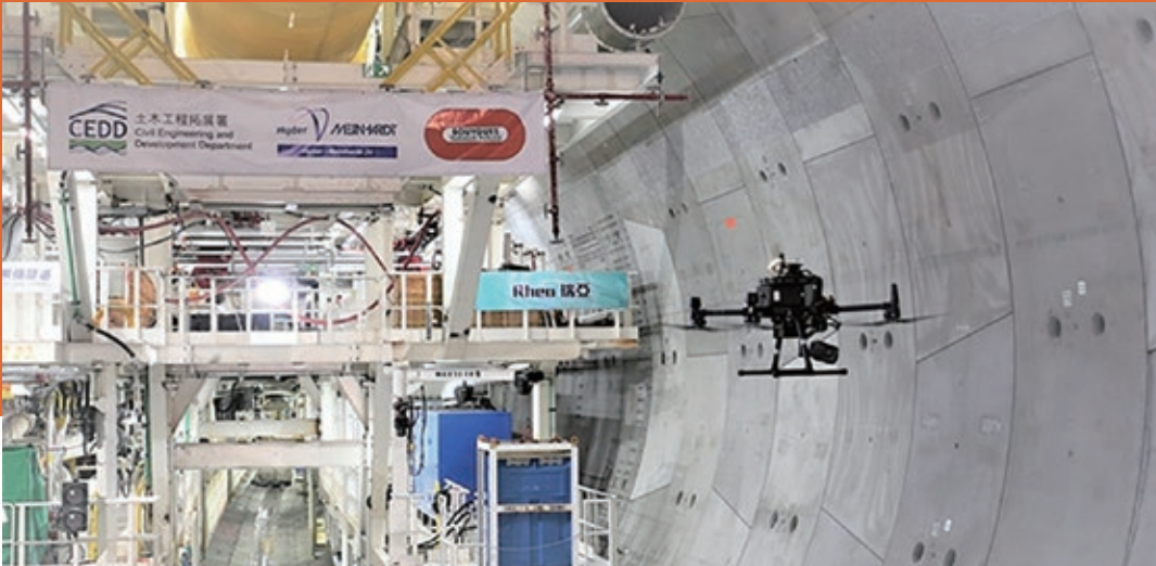
■ 運用邊緣人工智能及傳感器融合的智能隧道表面檢測系統 Edge-AI powered multi-sensor aerial inspector for tunnel surface
